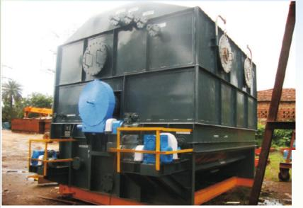
GAS TIGHT FILTER SIZE: 10' DIA X 10' LONG FOR OIL EXTRACTION FROM SPENT BLEACH EARTH (INDONESIA)
